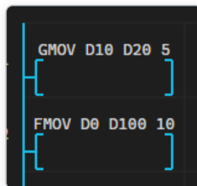
< Figure 6-20 A block transfer example circuit — GMOV D10 D20 5 and FMOV D0 D100 10 box functions placed with no contact >
