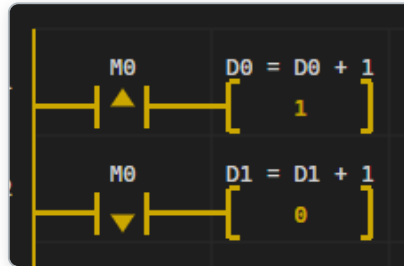
< Figure 5-16 A rising edge contact example — immediately after M0 turns ON, the contact conducts for that single scan and D0 increases by 1 >
