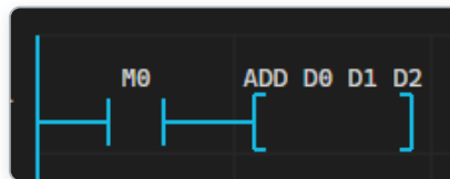
< Figure 6-14 A basic arithmetic ADD example circuit — the ADD D0 D1 D2 box function placed after an M0 NO contact >
