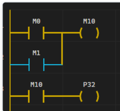
< Figure 5-4 A parallel OR example with NO contacts — if M0 or M1 is ON, P32 turns on by way of M10 >
