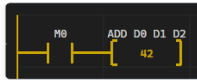
< Figure 6-15 ADD monitoring — the result of D0+D1 being reflected in D2 while M0 is ON >
